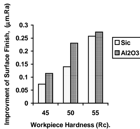
Fig. 8 Effect of Work piece hardness on Surface finish
