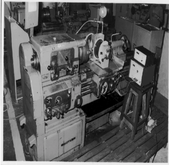
Fig 3. Machining setup developed for semi-magnetic abrasive machining
